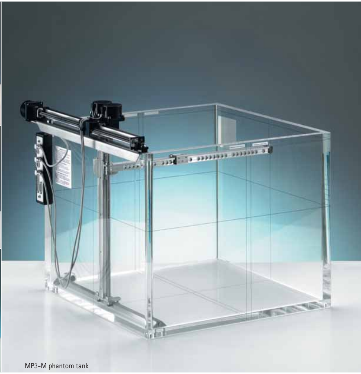
SCANLIFT carriage with positioning device
